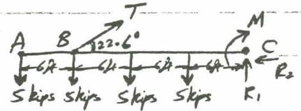
(a)  $T = 39 \text{ Kips} \therefore$  from (1)  $20 = R_1 + 39 \times \sin 22.6 \therefore R_1 = 5 \text{ Kips}$
