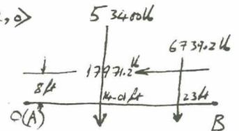
∴ (a) The reaction is  $\langle 17971.2, 60139.2 \rangle \text{ lb}$  at  $x = 12.63 \text{ ft}$
